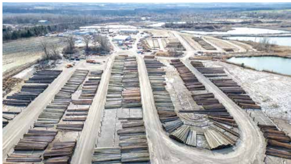
The Scottsville yard, with 394 pole bunks. The spoke-and-wheel design maximizes storage space.
