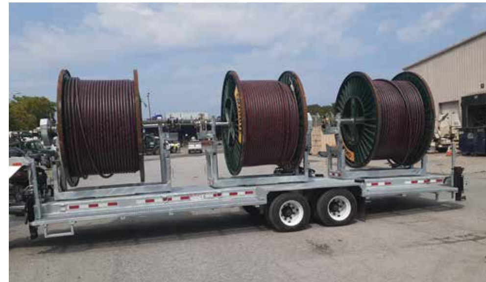
Our 2021 30,000-pound, three-ring cable trailer carrying three reels of 35-kV 750-mcm EPR cable
