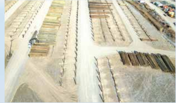
The Scottsville pole yard. Bunks are made using reclaimed poles retired from utility line support. Upright bunk support poles are typically 15 feet long and buried 4 feet deep.
